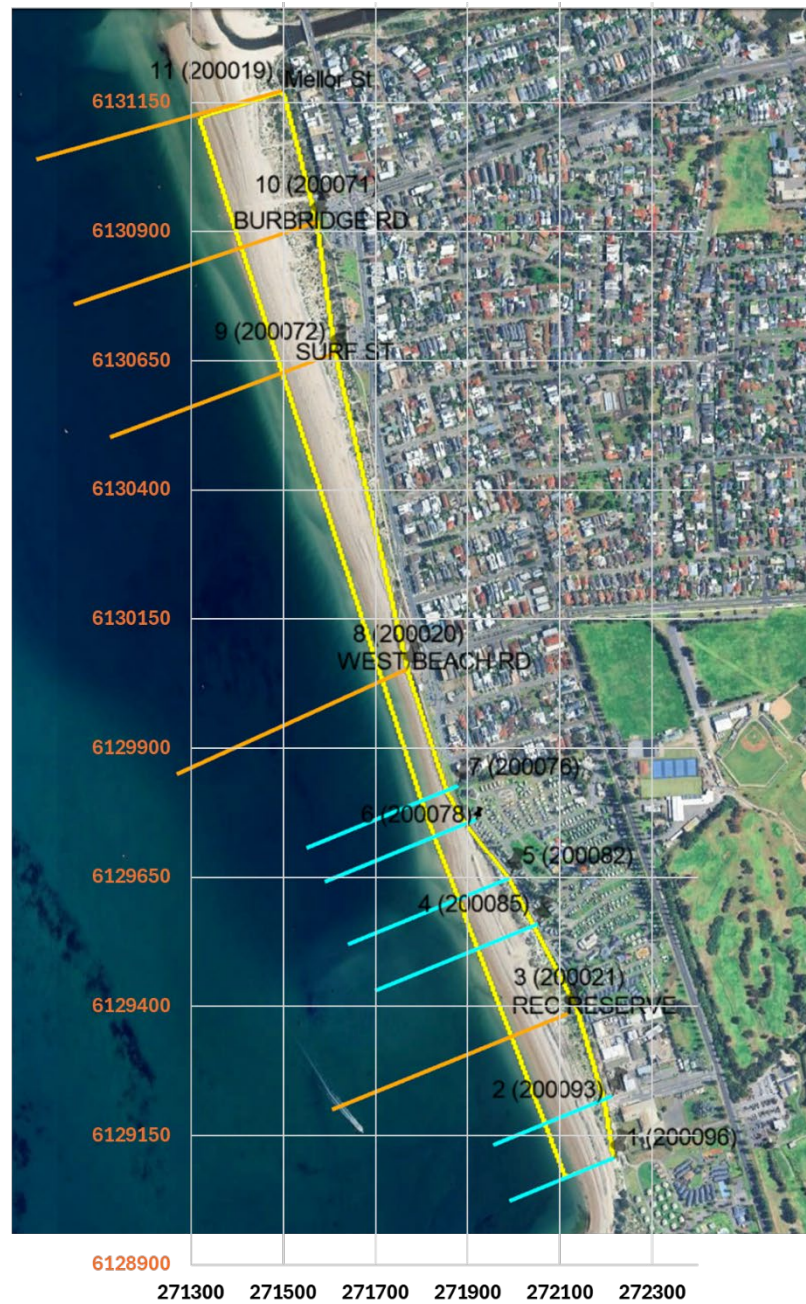
Figure 3-2 Cross-shore profiles locations and directions used for West Beach (Cell 3) sand volume study.
