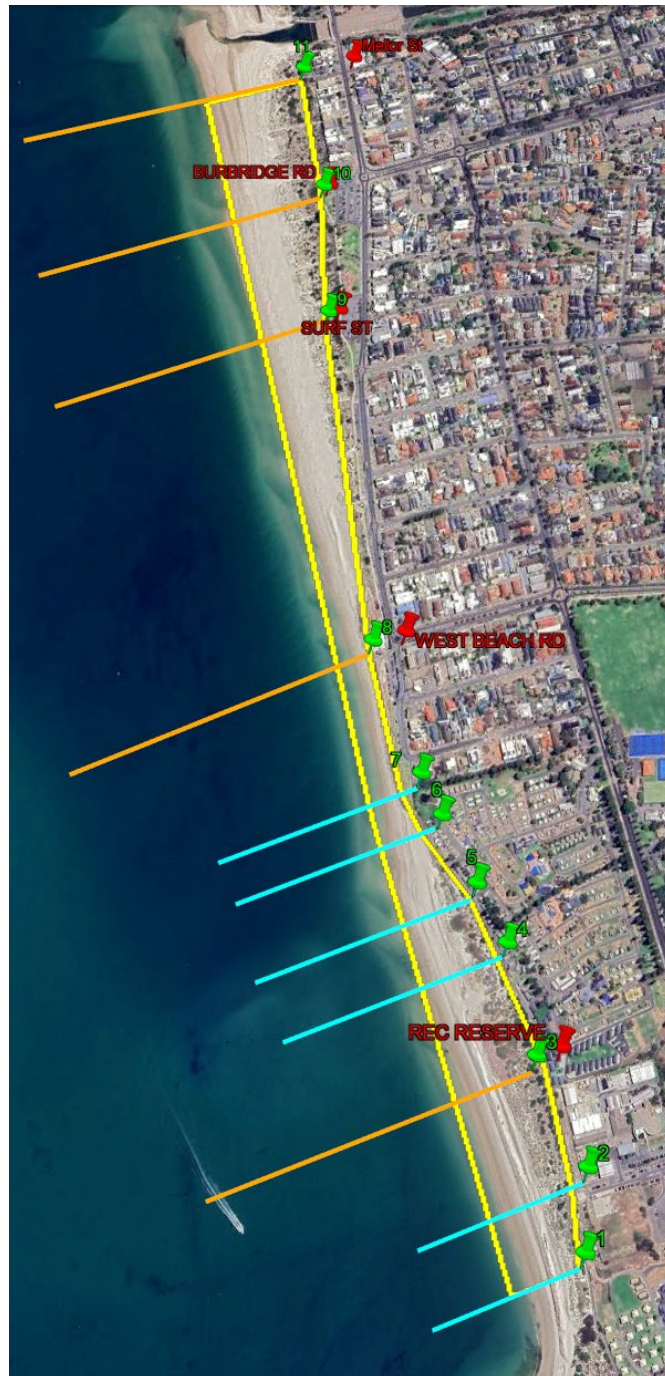
Figure 3-1 Locations and directions of cross-shore profiles surveyed for the West Beach zone (Cell 3).
