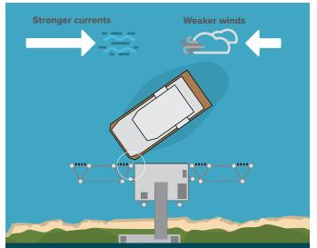
For winds blowing off the station, let the current and motor push the vessel onto the guide pile.
