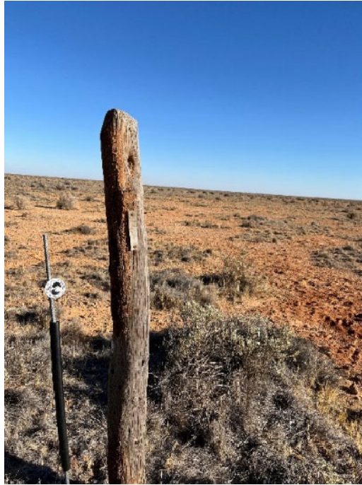
Example of marker peg (1971 mulga, 2024 reo rod and poly marker)
