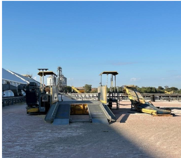
Belt conveyor along western side of paired sheds connecting storage to railway outloading bins (left) and a drive-over-hopper (right).
