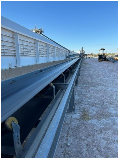
Belt conveyor along western side of paired sheds connecting storage to railway outloading bins (left) and a drive-over-hopper (right).
