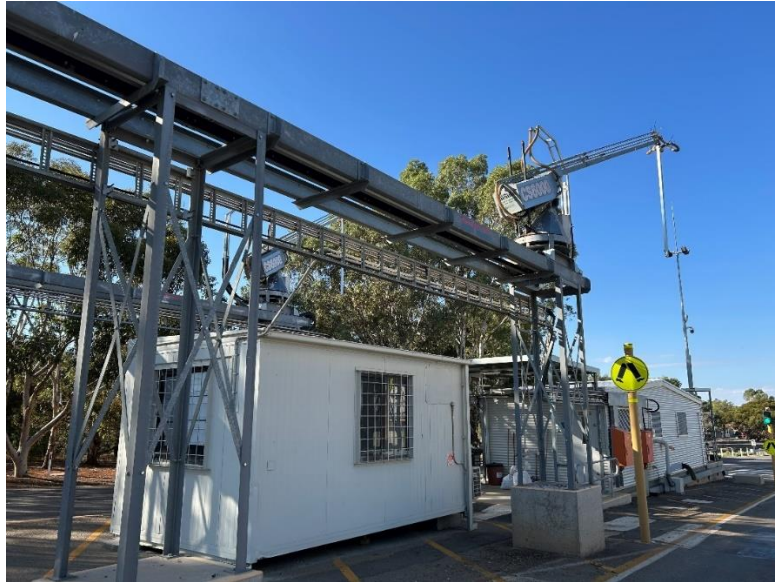
Classification centre with automatic grain probe system.
