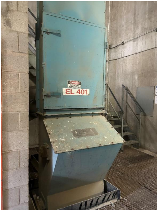
One of the grain elevators of the 24-cell concrete vertical silo (left) and the interior of the grain elevator.
