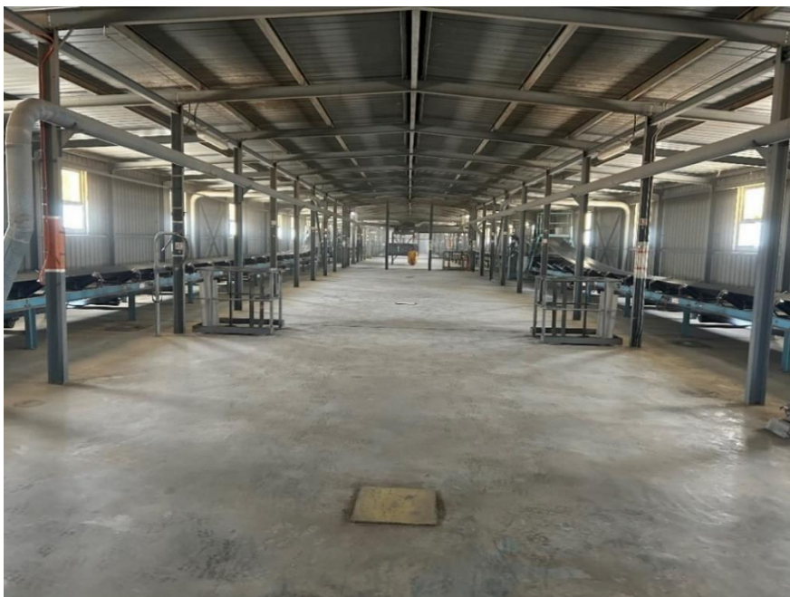
Interior of the grain conveyor enclosure at the top of the concrete vertical silo. The conveyor belts on either side feed the grain from the elevators into their allocated storage cell below.
