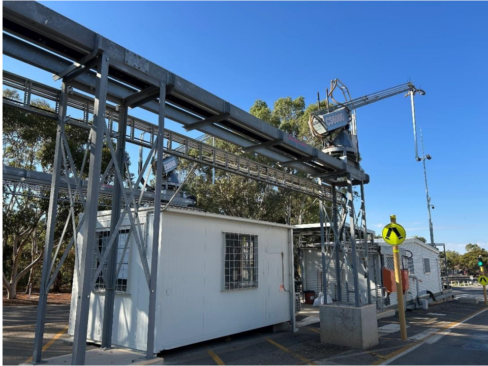
Classification centre with automatic grain probe system.
