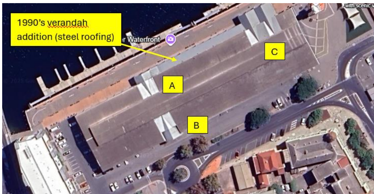
Figure B. Overhead view of Wharf Shed 1 showing 1990's veranda addition and lettered location of roof changes. Otherwise, the original 'Fibrolite' corrugated roof sheeting remains. Source Google Earth accessed 20/6/25.
