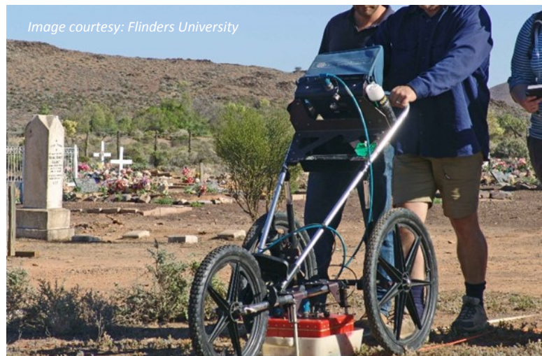
Remote sensing survey of land adjacent to a cemetery using GPR to locate unmarked graves
