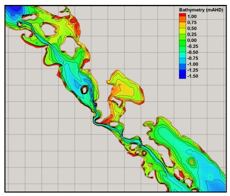
Figure A.2: Dredge Scenario Bathymetry through Hells Gate Area (Channel is typically 20m wide at -0.8 mAHD), Grid Size = 1000m
