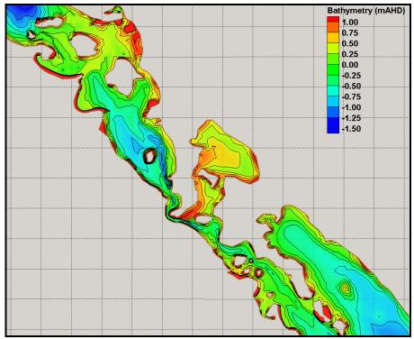
Figure A.1: Existing Bathymetry through Hells Gate Area (Base Case), Grid Size = 1000m
