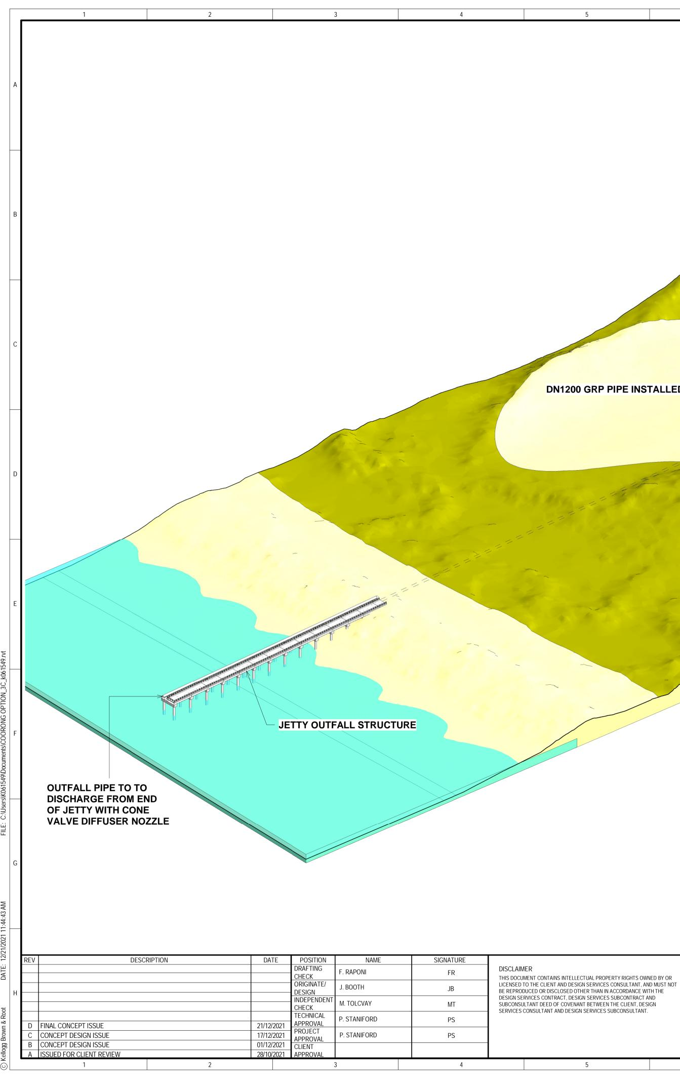
DN1200 GRP PIPE INSTALLED THROUGH DUNES
