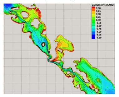
Figure 5: Modelled Bathymetry following Dredging (BMT WBM, 2009)
