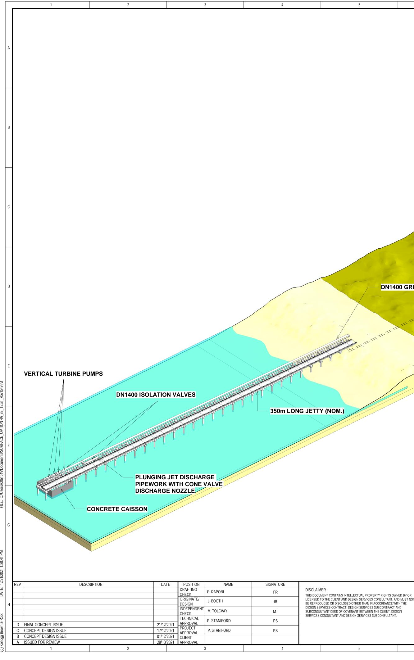
DN1400 GRP PIPEWORK INSTALLED THROUGH DUNES
