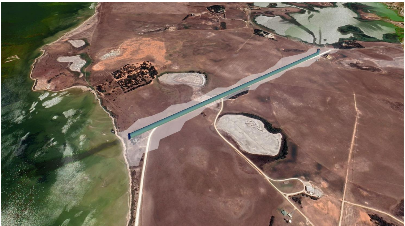
Figure 7 Visual representation of Concept 1B demonstrating the piped Lake Albert connector that would connect Lake Albert to the Coorong North Lagoon
