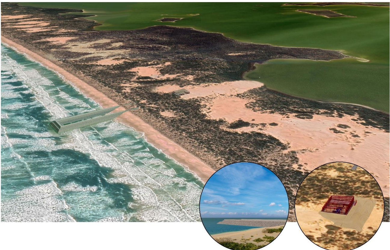
Figure 15 Visual representation of Concept 4A demonstrating a central pumping station in the Young Husband Peninsula and a breakwater at the Southern Ocean discharge
