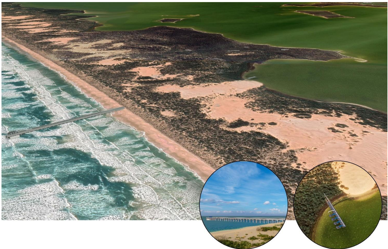
Figure 14 Visual representation of Concept 1A demonstrating the passive channel that would connect Lake Albert to the Coorong North Lagoon
