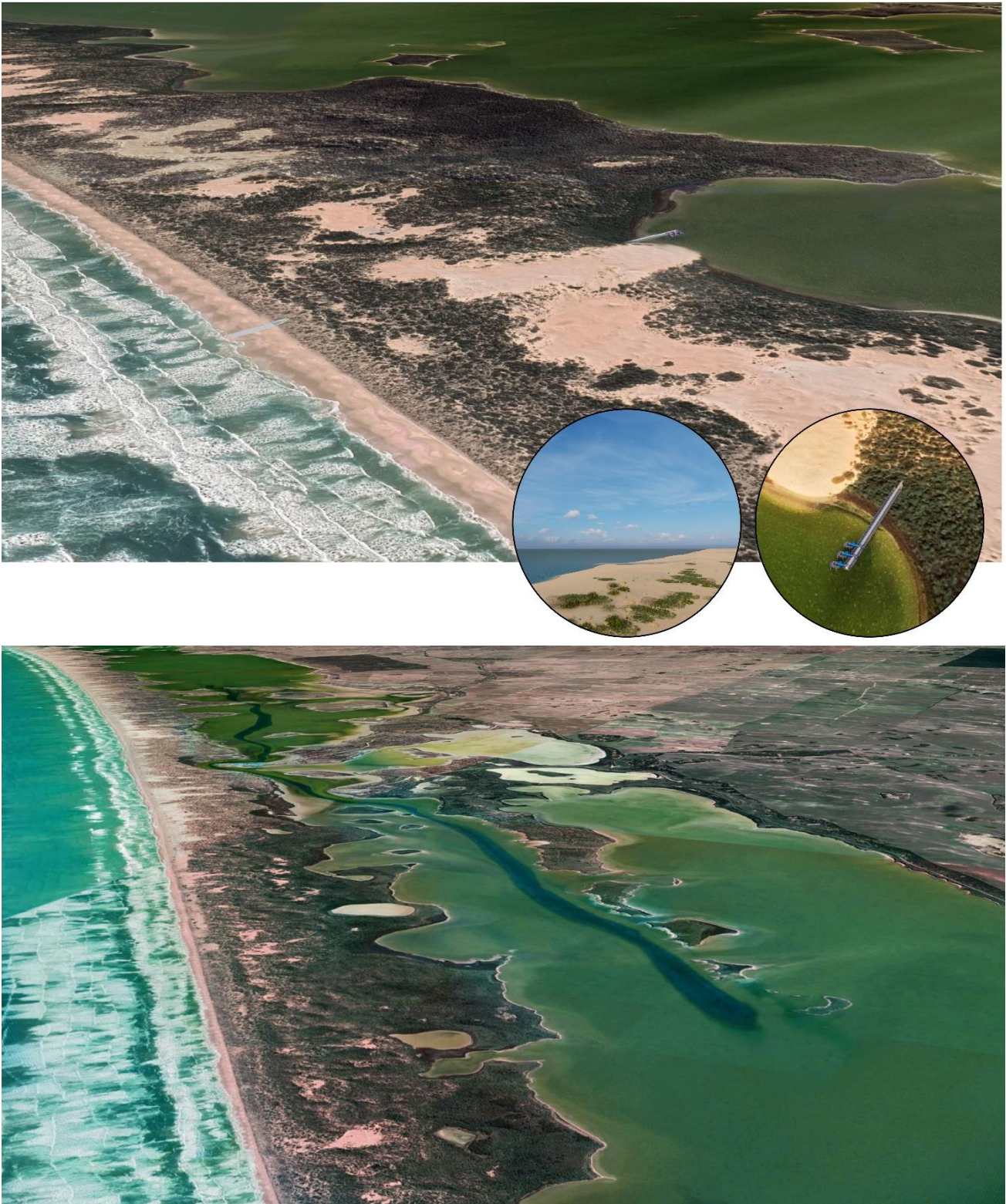
Figure 13 Visual representation Concept 3D demonstrating the pump out concept with a low visual impact FlexMat discharge into the Southern Ocean [top], and the 17.5km dredge alignment either side of Parnka Point [bottom]
