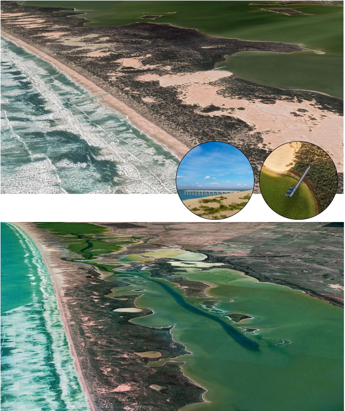
Figure 12 Visual representation Concept 3C demonstrating the pump out concept with a 150m jetty discharge into the Southern Ocean, and the 17.5km dredge alignment either side of Parnka Point
