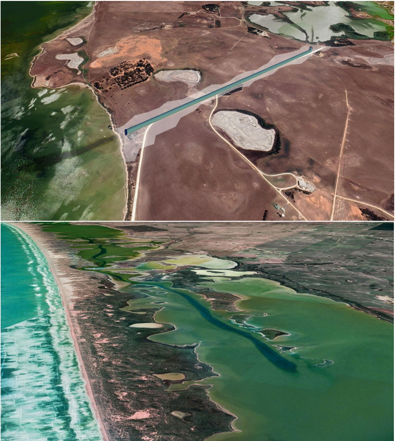
Figure 9 Visual representation of Concept 1B+2 demonstrating the piped Lake Albert connector that would connect Lake Albert to the Coorong North Lagoon [top] and the 17.5km dredge alignment either side of Parnka Point [bottom]
