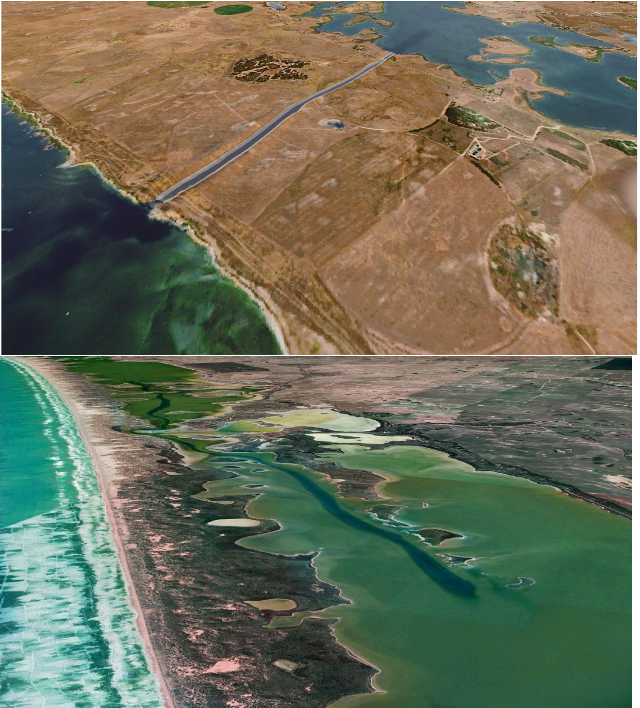
Figure 8 Visual representation of Concept 1A + 2 demonstrating the passive Lake Albert connector channel that would connect Lake Albert to the Coorong North Lagoon [top], and the 17.5km dredge alignment either side of Parnka Point [bottom]
