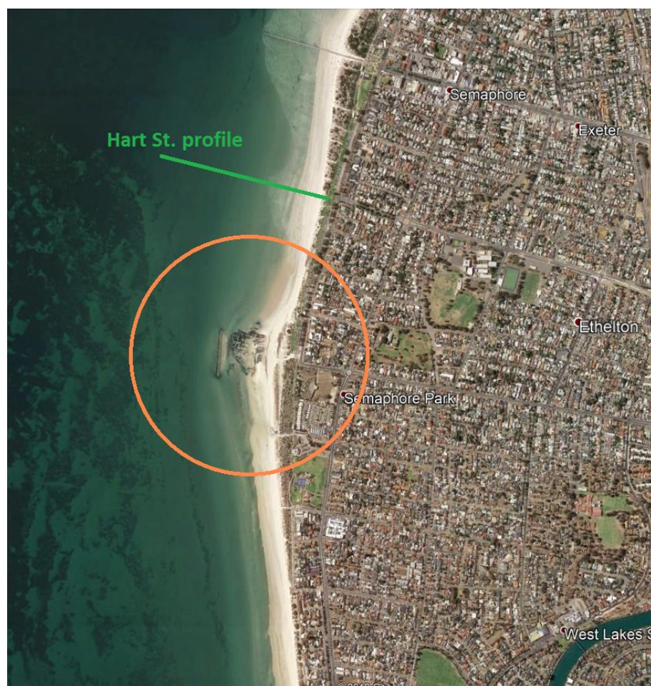
Figure 2.1 Offshore breakwater constructed in Semaphore in the late 1990s and location of the cross-shore profile presented in the figure below.
