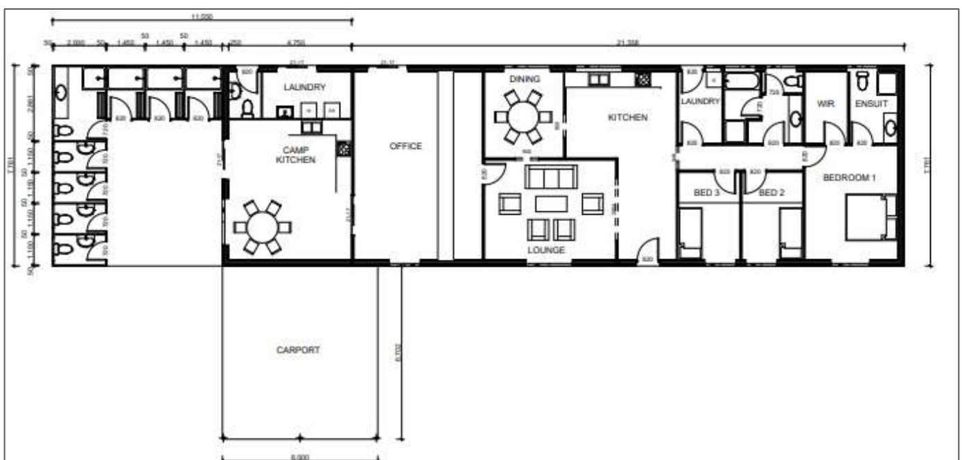
Figure 4. Schematic of the proposed caretaker residence which includes toilets, office and camp kitchen facilities, all under the main roof.
