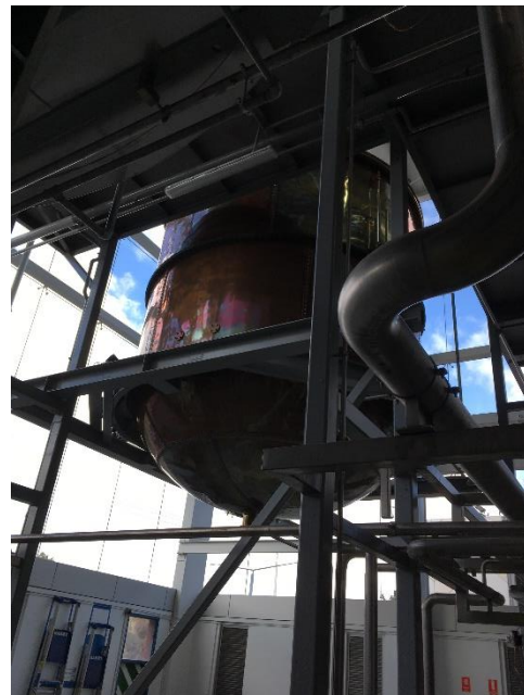
Copper kettle, showing riveting and rounded base.
